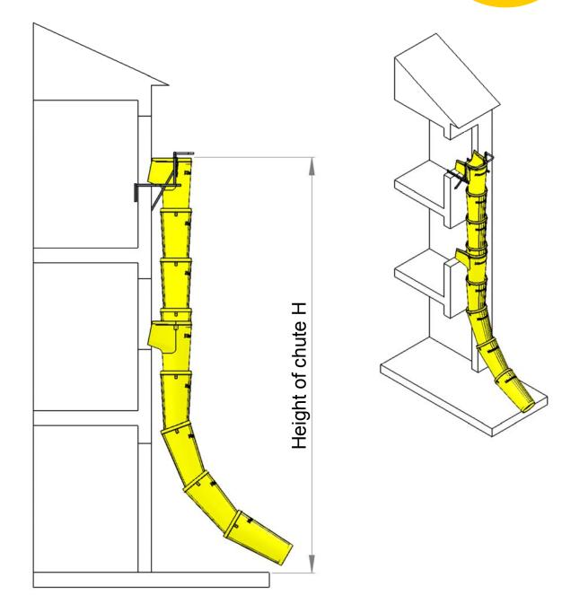
Overall length of a rubbish chute/hopper = 1,10mWorking length of a rubbish chute/hopper = 0,85mN = number of chute sections required for a height of chute H N = H/0.85 m (rounding up) To achieve an angle, add a supplementary rubbish chute.
