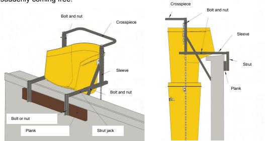
The chute sections can now be mounted to the window fixing frame.
