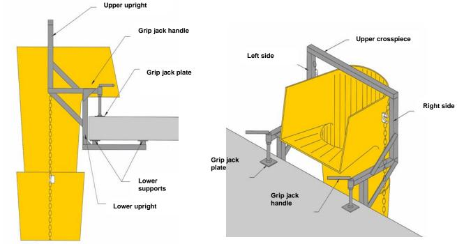
The chute sections can now be mounted to the platform fixing frame.
