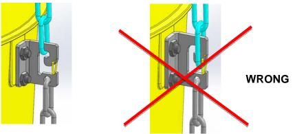
Anchor the rubbish chute to the building using a rope or a chain every 10m (30ft).
